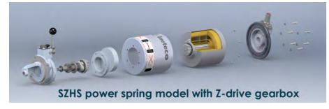
The user winds a spring in the starter using the supplied cranking handle and converts stored potential energy into rotational kinetic energy used to turn over and start the engine. The user can wind the ratched as fast or as slowly as they wish. Once wound, the spring starter can be tripped by pushing a trip lever on the starter when the user is ready and chooses to do so. Using a Kineteco spring starter is safe and easy.
