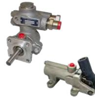
The KTI hand pump is a manual pump capable of regenerating system pressure for a starting attempt. Equipped with a 91 cm lever, the manual pump operates on "human" power and can recharge a hydraulic system in a black start condition, thus emphasizing yet another reason why it is relied upon in emergency starting applications.
