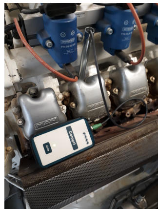
Compri installed on a power plant MAN E2842 Le312 4-stroke gas engine
