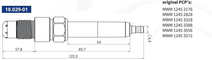
Alternative for all metal barrel PCP's currently suitable for the above mentioned engines.
